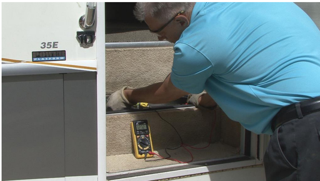
Checking battery voltage with a multimeter
